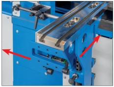
Movable front gauge with digital readout
