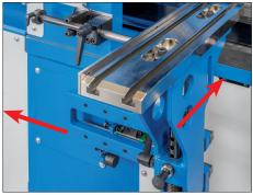
Movable front gauge with digital readout
