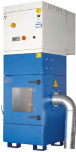
**Spark separator**, Temperature control and extinguishing device are standard
