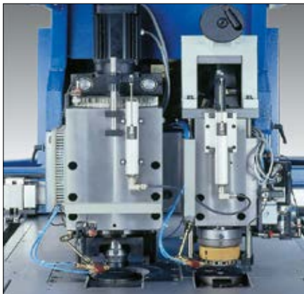
Solid construction of the punch heads with DC motor and measuring system
