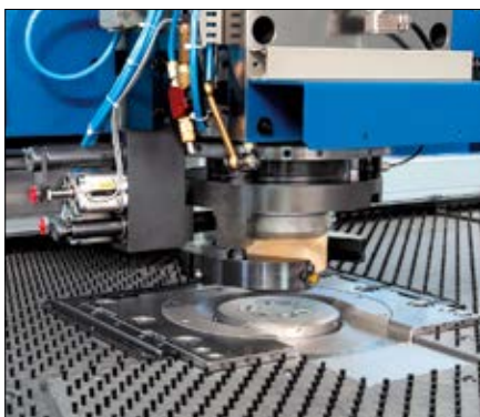
Punching head rotation Index equipment and also stripper height adjustment
