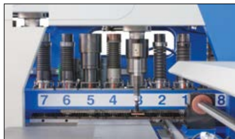
Optional threading from M3 to M16. Three thread diameters can be in operation simultaneously.
