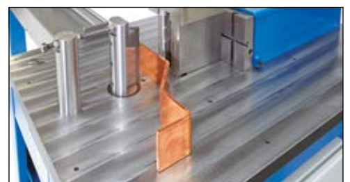
Messuring prism with automatic spring-back compensation and bending without marks for copper, aluminium and steel.
