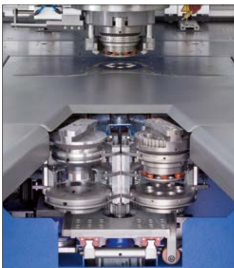
8 station tool carousel with cassettes that hold punch, die and stripper or Revotool head with 4, 6 or 8 tools.
