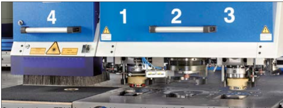
Combicut laser TRI 3-head punching machine with 2xRevotool (head 1 + 3) and rotation / index (head 2)
